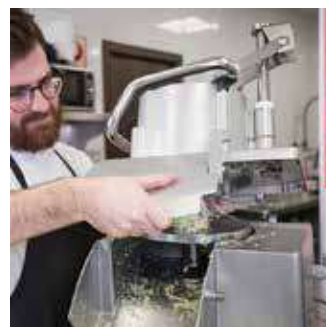
Lever and lid easily removable for cleaning purpose.
